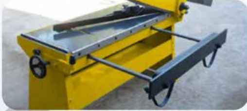
Çift Kramyerli Arka Dayama Double Gear-rack Backgauge
